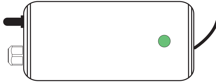
Green LED indicates UV lamp “ON”.
